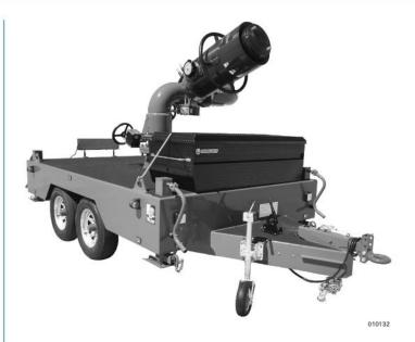
Highly Efficient Waterway – The trailer has a 12 in. (300 mm) integrated stainless steel waterway to provide minimum friction loss, maximum efficiency, and reliability. The inlet manifold features standard Storz couplings with caps. Various combinations of inlet sizes are available to provide maximum connectivity. The monitor is built with a 10 in. (250 mm) waterway. The nozzle features a hard coat anodized aluminium and stainless steel assembly.
